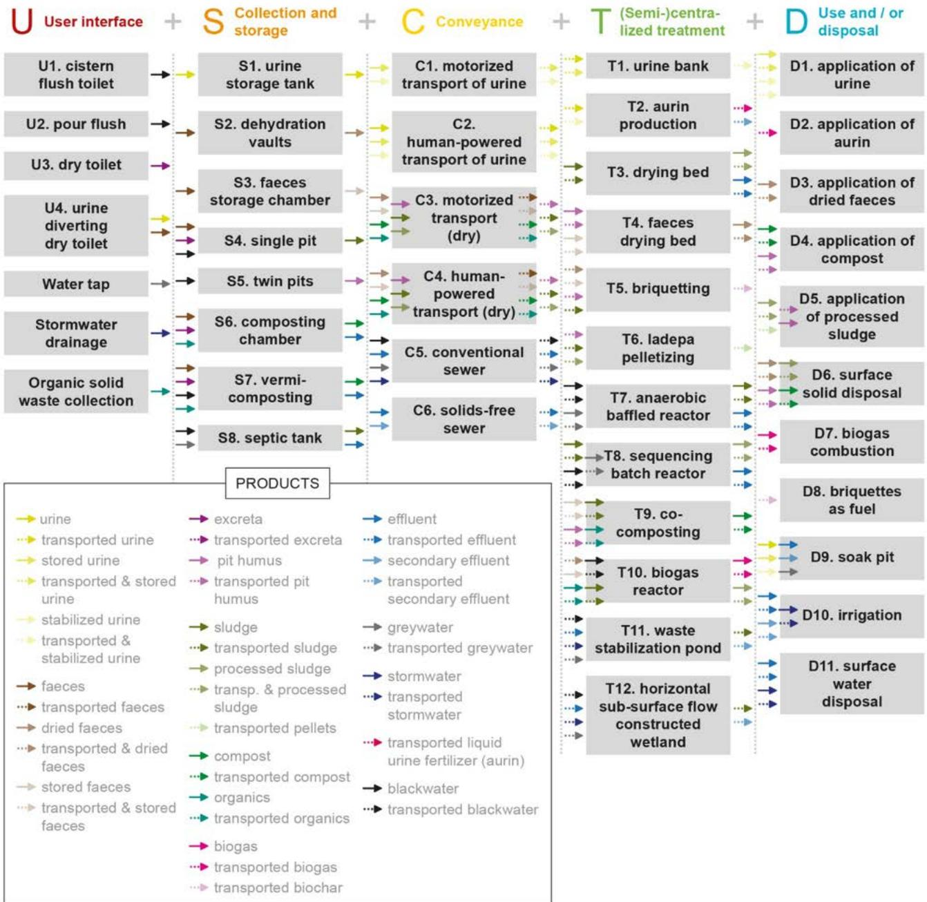
Figure 4.6: Overview of the set of sanitation technologies currently available in the technology library for five functional groups. Each box represents a technology. The arrows represent the input and output products. So far only toilet sources are implemented, although greywater, stormwater, and organic waste sources can also be considered by the model.
