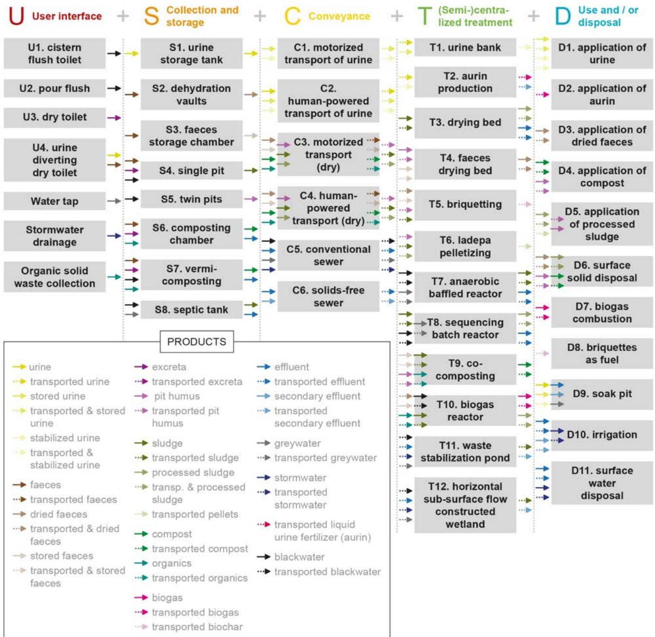
Figure 5.2: Overview of the 41 technologies in this study used to generate sanitation systems and to quantify their substance flows grouped by functional group. Each technology is defined by its name, possible input and output products, and how these products relate to each other (e.g. 'OR' for either one or another, 'AND' if they always arise jointly). Taken from Spuhler et al., (2020c).
