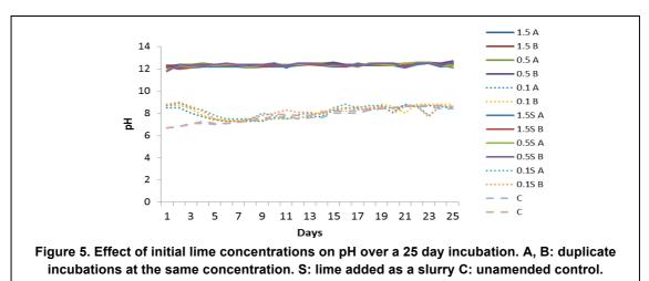
In comparison with the control and 0.1 % of lime amendment, addition of 0.5 and 1.5 % of lime followed by thorough mixing, resulted in an almost instantaneous precipitation of solids to the bottom of the containers, and the formation of a clear supernatant. A distinct ammonia odor was detected. This odor
