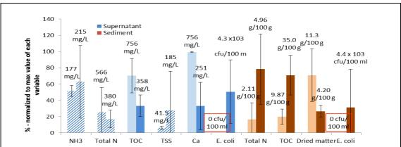
Figure 6. Characteristics of supernatant and sediment after incubation. For each parameter, the left column is average of high lime-amended ("high treatment", 0.5 and 1.5 % w/v lime) incubations and the right column is average of control and amendment at 0.1 % (w/v) lime ("low treatment). Hashed columns are not significantly difference. Solid fill represents difference at p(same) < 0.05.
